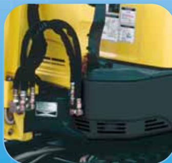
Careful routing of hydraulic pipes and hoses
