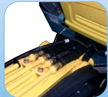
Hydraulic hoses pass in the center of the upper frame : perfect protection and no twisting
